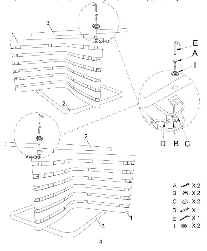
Step 4. NOTE: It may be necessary to apply pressure and force to place back and seat (part #1) into position. Attach support legs (parts #2 & #3) to back (part #1) using bolts (part A), flat washers (part C), round plastic washer (part I), plastic washers (part G), nuts (part B), wrench (part D) and allen key (part E). Please fully tighten all bolts.
